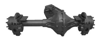
Heavy duty drive axle with high capacity disk brakes.
